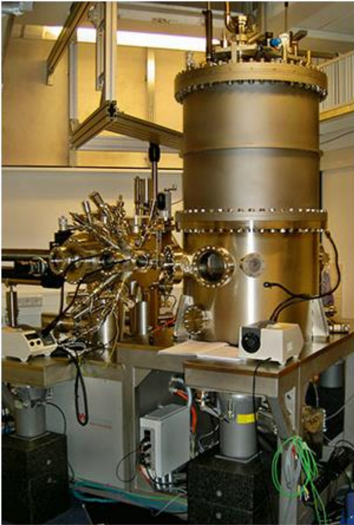
➤ Home built 4K-STM with 3D Magnets
